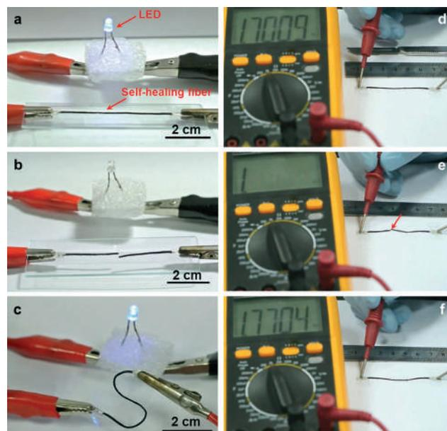
**Figure 5.** a,b,c) Photographs of a self-healing fiber serving as a conducting wire to power a LED before breaking, after breaking, and after healing and being bent, respectively. The voltage was set at 3.2 V. d,e,f) Electrical resistance of a fiber with a length of 5 cm before breaking, after breaking, and after healing, respectively. The red arrow in (e) indicates the breaking position. The unit of the resistance displayed on the multimeter was  $\text{k}\Omega$ .
