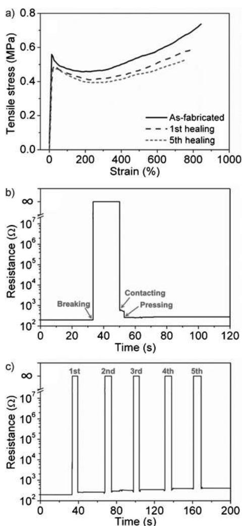
**Figure 4.** Mechanical and electrical properties of the aligned-CNT/SHP fiber before breaking and after healing. a) Stress–strain curves of an as-prepared fiber and the fiber after one and five cycles of breaking/healing. b) Electrical resistance of a fiber before breaking, after breaking, and after healing. c) Electrical resistance in five breaking/self-healing cycles.
