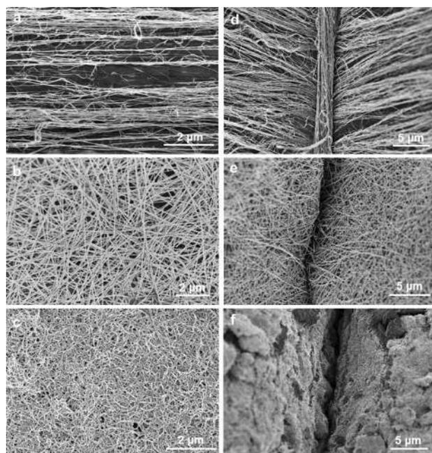
**Figure 2.** SEM images of three self-healable fibers. a,d) A CNT-sheet-based fiber before breaking and after self-healing, respectively. b,e) A silver-nanowire-based fiber before breaking and after self-healing, respectively. c,f) A CNT-network-based fiber before breaking and after self-healing, respectively.
