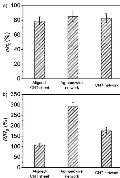
**Figure 3.** Comparison of the mechanical and electrical properties of three conducting wires after self-healing. a) Tensile strength:  $\sigma_0$  and  $\sigma$  correspond to the strength before breaking and after self-healing, respectively. b) Electrical resistance:  $R_0$  and  $R$  correspond to the resistance before breaking and after self-healing, respectively.
